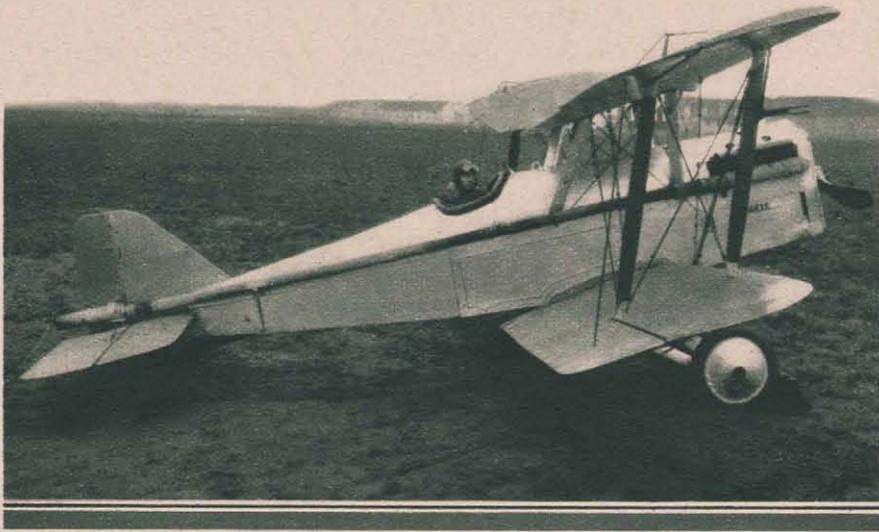
*This is what might be called a "sky pen." It is the plane that is used in spelling out words in a white chemical smoke 10,000 feet in the air. The exhaust pipe through which the smoke passes can be seen running along the side of the fuselage.*
